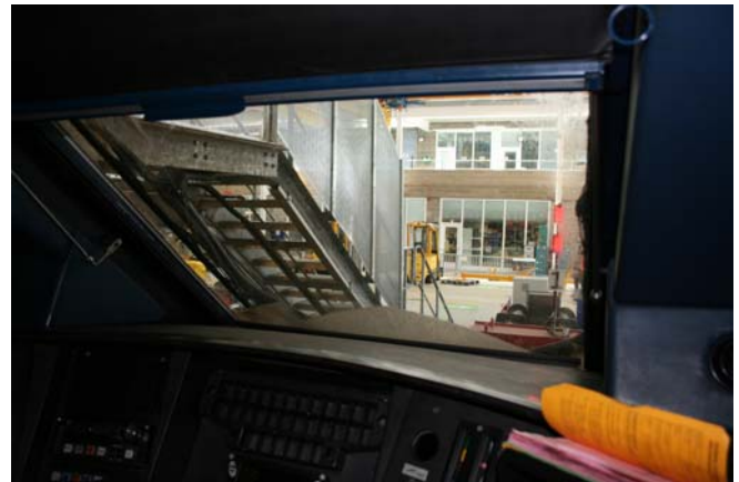
The View from the Driver's Seat. (Designed to provide a blinkered view, concentrating the driver's eyes on the way ahead, and to avoid stroboscopic problems.)
