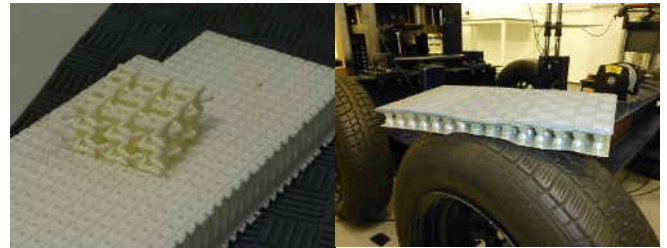
3D printed 'blast mats' fitted to the floor of military vehicles to reduce the transferred impulse in order to reduce the risk of injury
