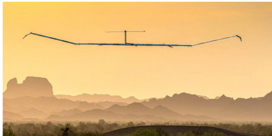
Fig 3: The Zephyr UAV. The 150lb aircraft, with an 80ft wingspan, operates in the stratosphere at an altitude of 70,000ft. AIRBUS
